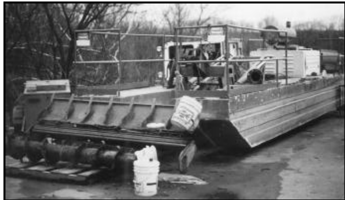
Figure 6. M-NCPPC's Hydraulic Dredge (a.k.a., Mud Cat) Used For Removing River Sediment.
