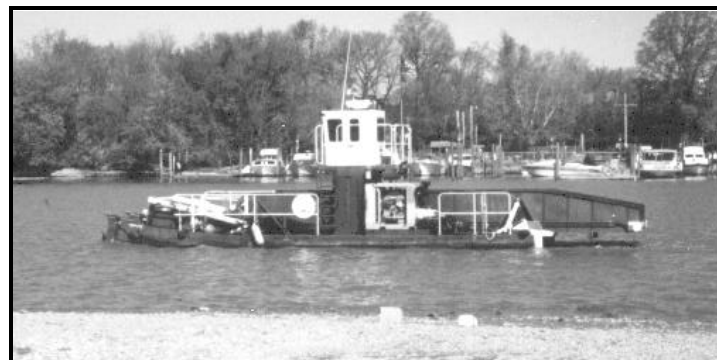
Figure 14. District of Columbia Trash Skimmer Boat Removing Floating Trash (photo: DC WASA, 1993).
