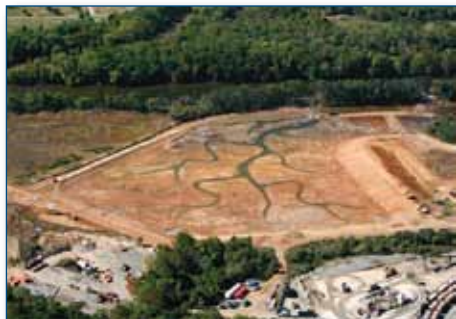
Figure 1-11: Tidal wetland restoration at Anacostia East Mitigation Site 11 for the Woodrow Wilson Bridge Project (M-NCPPC and Prince George’s County)
