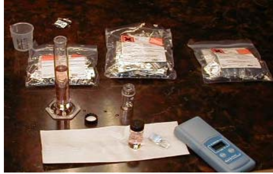
Figure 16. Sample Rain Barrel Water Quality Testing Equipment
