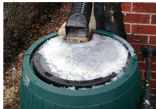
Figure 15. Ice Accumulation on Rain Barrel Screen
