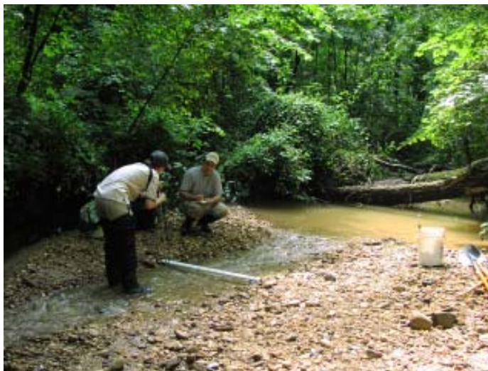
Figure 4 - Lower reach - COG Staff Measuring Baseflow
