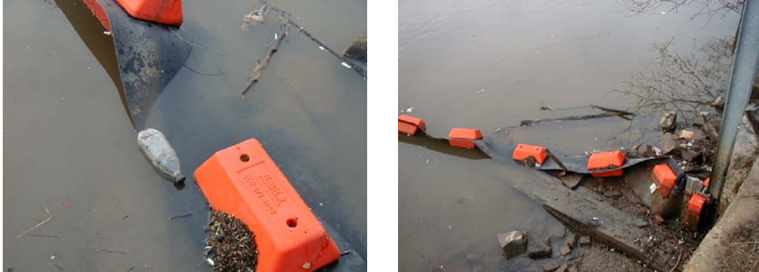
Figure 30. Floatables Breaching Flexible Floating Boom During Low Tide
