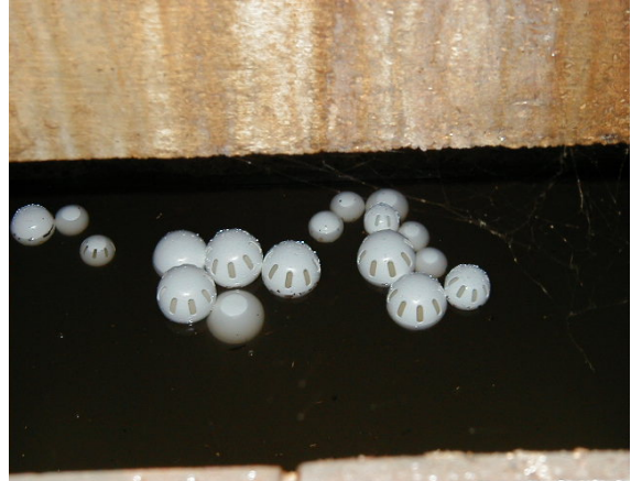
Figure 14. Mark-Recapture Balls Following Release into CSO 018 System
